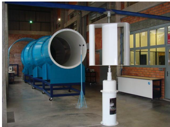
Fig. 4 Vertical axis wind turbine testing in wind tunnel
